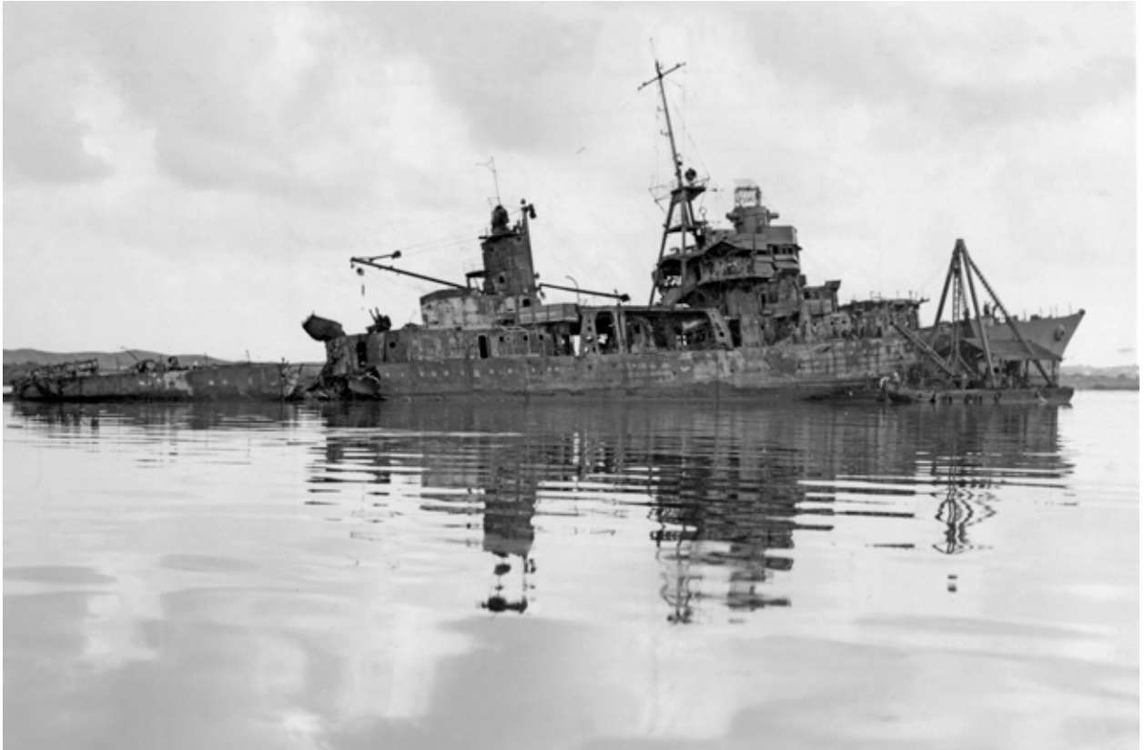
Photo 1: ERIE (PG 50) General view of torpedo and fire damage from off starboard quarter.
